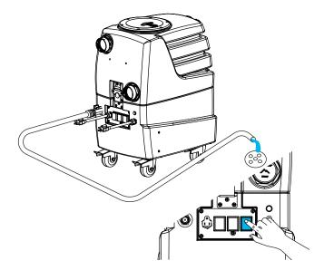
The recovery tank can be emptied using the pump-out feature. Attach a garden hose to the pump-out fitting, place the other end of the hose in a drain or receptacle, and press the PUMP-OUT switch on the switchplate. •
