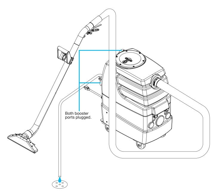
The Air Hog™ does not have a solution tank or solution pump. However, it can be used to extract pre-sprayed solution from carpet.
