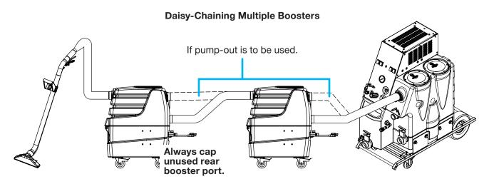
If the pump-out will be used, connect vacuum hose from extractor to top rear booster port and cap the bottom one. If not, connect hose to the bottom rear booster port and cap the top one. Recovered water will flow through the Air Hog<sup>TM</sup> to the extractor.
