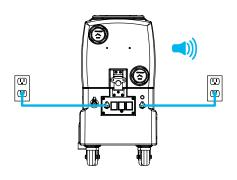
Each power cord on the Air Hog<sup>™</sup> requires a grounded 15 amp outlet. The dual circuit indicator light and tone will activate when this is achieved. ◆
