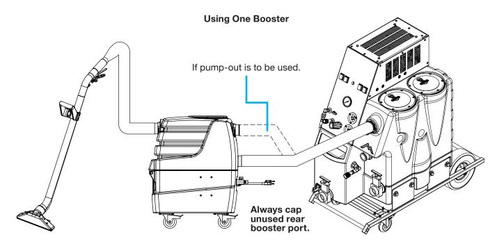
If the pump-out will be used, connect vacuum hose from extractor to top rear booster port and cap the bottom one. If not, connect hose to the bottom rear booster port and cap the top one. Recovered water will flow through the Air Hog<sup>TM</sup> to the extractor.
